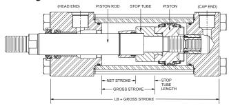
When specifying cylinders with long stroke and stop tube, be sure to call out the net stroke and the length of the stop tube. Machine design can be continued without delay by laying in a cylinder equivalent in length to the NET STROKE PLUS STOP TUBE LENGTH, which is referred to as GROSS STROKE.
